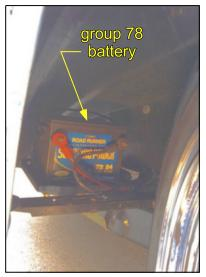
Battery is located behind right front wheel splash shield.
