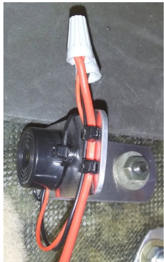
Buzzer strapped to aluminum bracket mounted inside firewall using front brake reservoir bolts.
